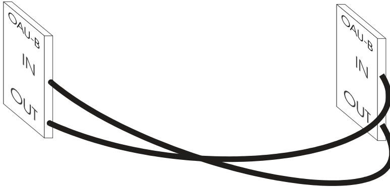
Figure 3 Start-up with one fiber pair and one OAU per NE
