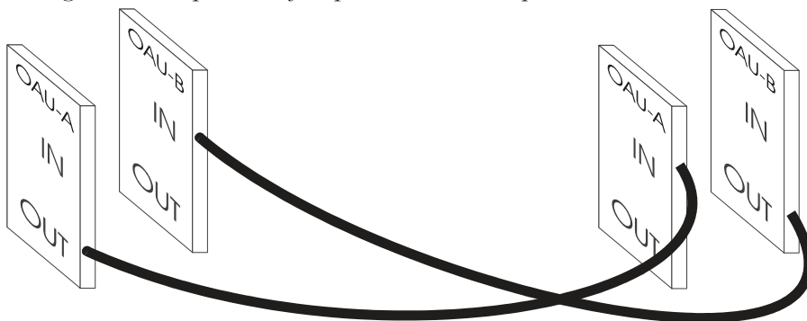
Figure 4 Start-up with one fiber pair and two OAUs per NE
