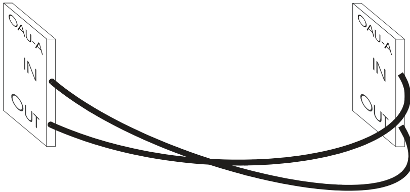
Figure 2 Start-up with one fiber pair and one OAU per NE
